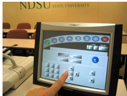
4. Choose the camera —classroom, instructor, doc cam, etc... Use the arrows to pan/tilt and zoom cameras
