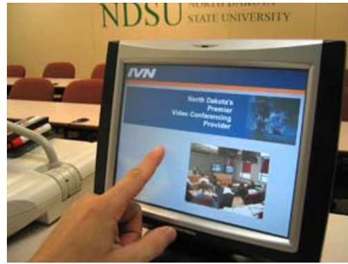
2. The panel may be on the ND-IVN home screen. Press anywhere on this screen to enter control screen
